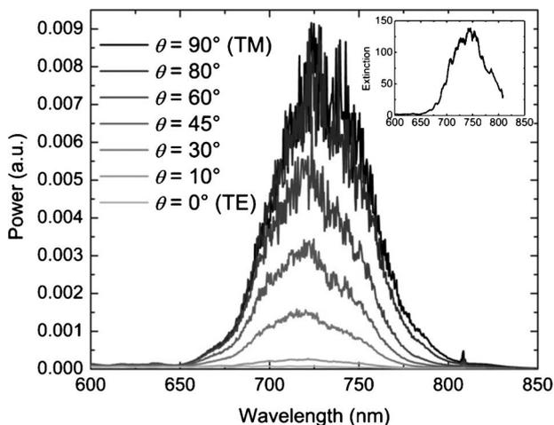
FIG. 4. Nonnormalized polarization dependent transmission spectra of a slit and groove structure on detector. The structure is that which has  $p=600 \text{ nm}$ . The inset shows the spectrum of the extinction ratio.
