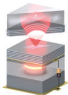
Figure 18: Sketch of a room temperature single photon source for quantum communication protocols. A quantum emitter (such as a defect in hBN) couples to the open cavity, enhancing the single photon emission.
